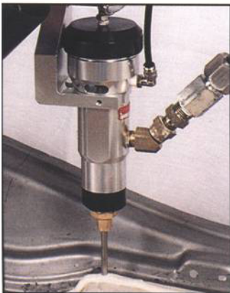
Dispensing Extruded Bead with 2200-033 Snuf-Bak™ Valve
